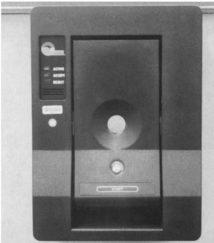
Figure 12-6. Iris scan device. The user aligns the eye with the camera in the center, then waits for a scan to be completed and to be granted access.
